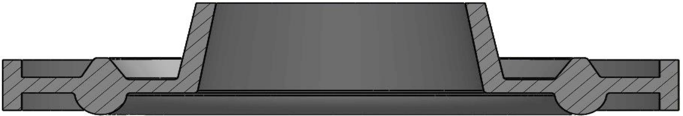
SPLIT VIEW – SEPTIC TANK SEAL
